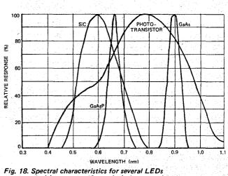
compared with response of a typical phototransistor.
