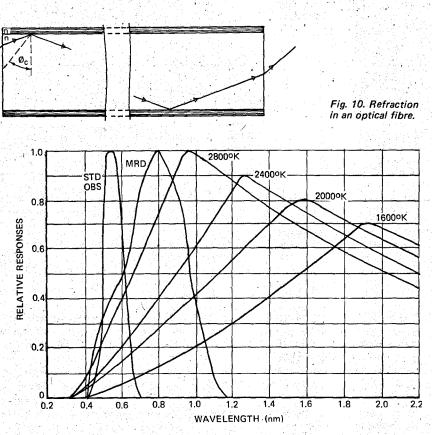
Fig. 11. Radiant spectral distribution of a tungsten lamp.
