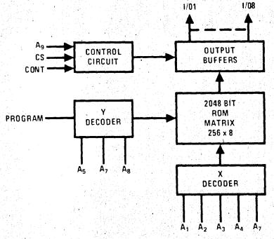
Fig. 1. Block diagram of National MM4203/MM5203 ROM
