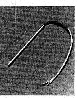
Thermistor protected by metal sheath operates to 300°C.
