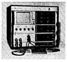
The General Radio RF Network Analyzer model 1710 provides precise measurements of transmission and reflection properties (including magnitude, phase, group delay, and S-parameters) over a broad frequency range of 400 kHz to 500 MHz. It also features, it is claimed, a full 115dB dynamic range, 0.005dB resolution, and the ability to operate into 50 or 75 ohms, without performance degradation.
