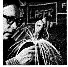
A new transmission concept is being examined by the British Post Office which employs laser beams to carry telephone calls along glass fibres. The principle behind it is that since the frequency of light is so much greater than that of a radio wave the potential information capacity of a light beam is correspondingly greater.
