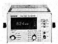
The Boonton Model 93AD True RMS Digital Voltmeter measures  $300\mu$ V to 300V in 12 programmable ranges of 1mV to 300Vfs. Frequencies from 10Hz to 20MHz are covered with a claimed accuracy of  $\pm 1\%$  rdg  $\pm 1$  digit over a large portion of the frequency band.
