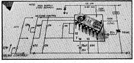
The IC1436 is a flexible integrated circuit providing phase controlled triggering of silicon controlled rectifiers and triacs. In addition, it contains an operational amplifier for use in closed-loop control or zero crossing switching applications.
