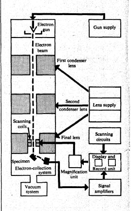
Fig. 14. Block diagram of Cambridge stereoscan electron microscope.
