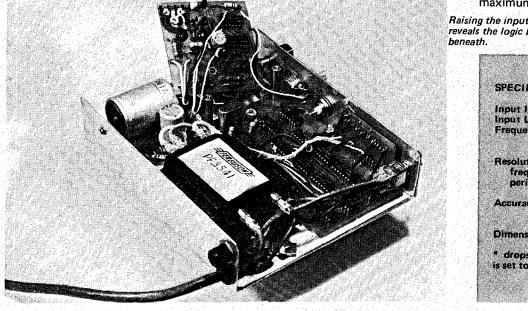
Raising the input board reveals the logic board
