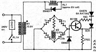
Fig. 4. Basically similar to Fig. 3, this circuit can handle relay operating coll currents of up to six amos.
