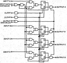
Fig. 2. Logic diagram of TRI-STATE quad flip-flop type DM8551
