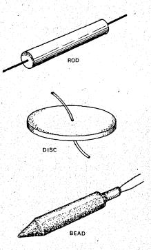
Construction of various types of thermistors
