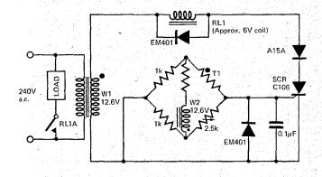
Fig. 3. Versatile low-cost controller.
