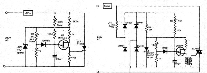
Fig. 9. Half-wave phase control system.
