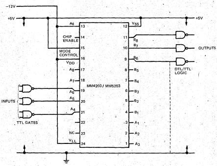
logic makes the device a very versatile Fig. 2. ROM connections and typical application as 256x8 PROM with TTL intertace.
