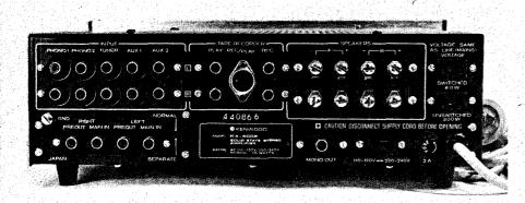
The amplifier has a few unusual performance characteristics. Firstly, the loudness control exhibited a response that was somewhat less than ideal. Over most of the range the response was normal, but at the maximum volume setting (and with a low level input) the treble response was cut and the bass response flattened out.
