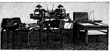
Fig. 13. This machine complex is used to plot maps and other contours from a stereo pair of photos.
