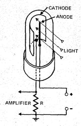
Fig. 1a. Photo-emissive vacuum-tube diode.
