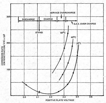
Fig. 5. Typical corrosion rate versus plate voltage per nickel-cadmium cell. The positive plate voltage is with reference to cadmium and the total cell voltage is the sum of the positive and negative plate potentials.
