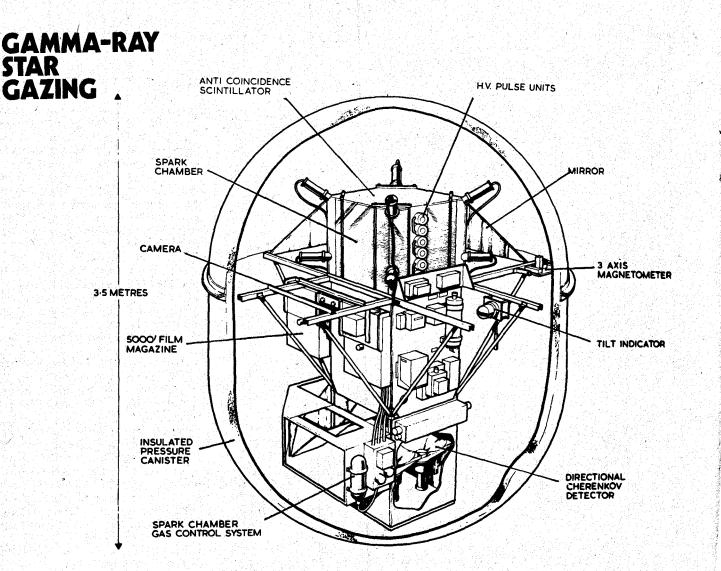
Fig. 3. This schematic drawing shows the contents of the insulated pressure canister used to house the guidance and measurement systems.
