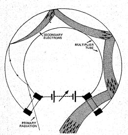
Fig. 5a. Curved tube improves electron multiplier operation.
