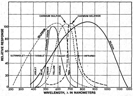
Fig. 7. Typical photodetectors - comparison of spectral responses.
