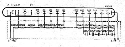
Fig. 3. Power supply divider chain for photomultiplier.
